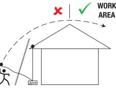
Test connection, move adjuster to knot end and throw to opposite side (use of throw line and sandbag is recommended)
