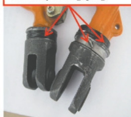
CORRECT FITTING Ball Bearings – Retained by a grub or slot head screw and covered by a strong spring
