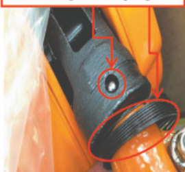
INCORRECT Ball Bearing + Weak Spring
