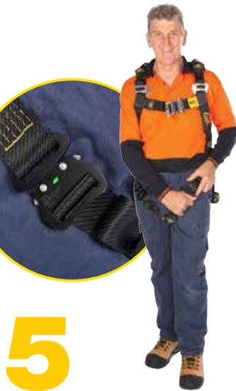
Bring leg straps between legs in turn ensuring no twist and connect respective strap to buckle on same side. Adjust by squatting and pulling on free webbing - repeat for both sides. Correctly fitted a flat hand should pass between webbing and leg BUT not a fist.
