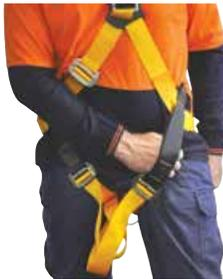
Correctly fitted, a flat hand should pass between webbing and leg BUT not a fist. If you can make a fist, tightening is required.
