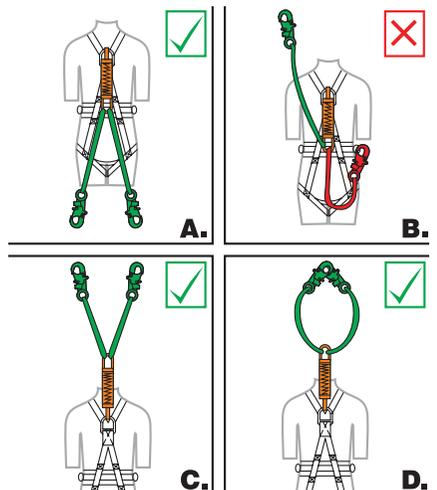
If you are using a B-Safe Twin Leg Lanyard, you must not attach the unused leg to anything other than the designated attachment/ stowage point.
